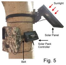
supplied to the camera. Now, the system start to work on duty at 24/7 and no longer worry about your device is running out of power. It will stay in the field to work as long as you want.
