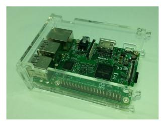
Place the above assembly around the Raspberry Pi and line up the slots.
