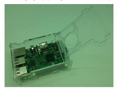
Attach the lid by inserting one post into the hole at the top, and then gently guide the other post into the corresponding hole, making sure the long slot in the side of the top plate lines up with the GPIO header. The lid can then be pivoted closed.
