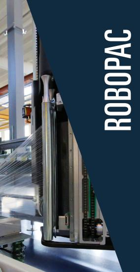
A key part of the installation is a Robopac Genesis HS50 high-speed rotary ring pallet stretch wrapper, using Cube Technology™ for precise use of film, position and containment force.
