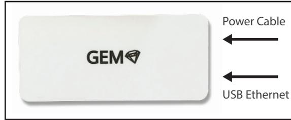
**STEP 2** Connect the Internet Bridge's Ethernet adapter port to a 'LAN' port on the back of your internet connected router using the patch cable supplied. Proceed to power up the Internet Bridge by plugging in the MicroUSB power supply. The Internet Bridge will take approx 90 seconds to boot.
