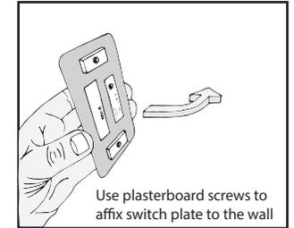
Screw the switch plate to the wall with two small plasterboard screws. **IMPORTANT - Use the included plastic spacers behind the switch plate. These provide the necessary spacing between backplate and wall.**
