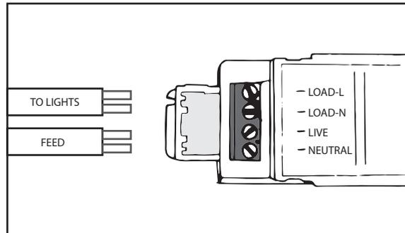
The connected lights should be wired in parallel with connection to the mains via the controller. Ensure the controller's maximum rating for a string of lights is not exceeded (500W ON/OFF; 100W Dimmable).
