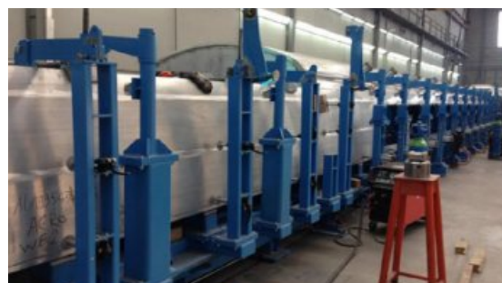
Welding and assembly fixture adjustment
