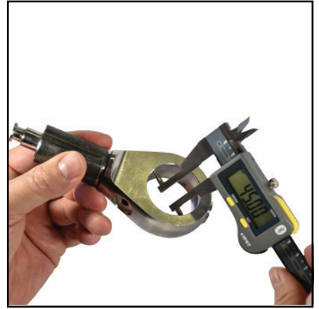
Internal measurement with S_Cal EVO BT PJ
