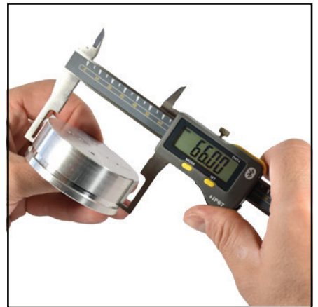
External groove measurement with S_Cal EVO BT EG
