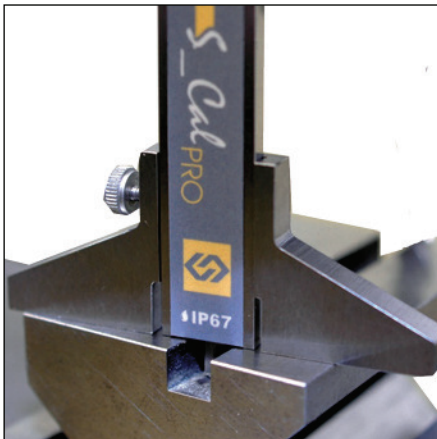
Depth measurement with S_Cal PRO and base 910.2205.
