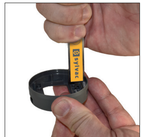
Depth measurement with S_Cal EVO \mu\text{m}
