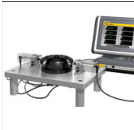
Multi-gauging measurement using D200S interface and D300S display
