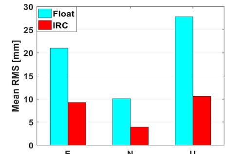
Fig. 4 Mean RMS values of PPP after convergence with IRC and Float solutions
