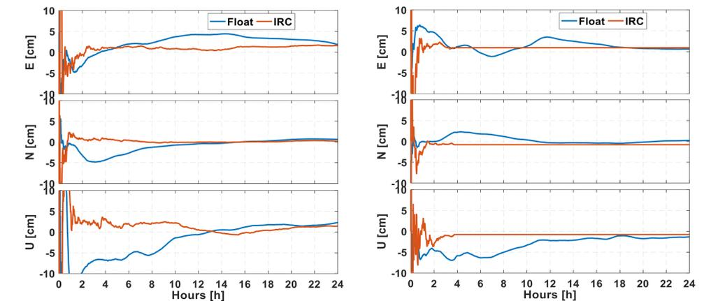
Fig. 3 Positioning performance of static PPP (BRAZ and ROAP station, DOY 106, 2017).
