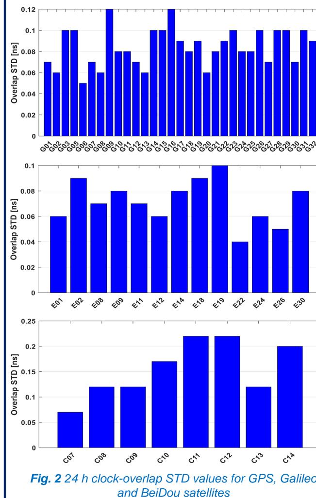
Fig. 2 24 h clock-overlap STD values for GPS, Galileo and BeiDou satellites
