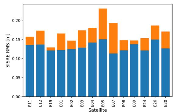
Figure 2 : SISRE RMS results of Galileo satellites for the period January 1st until June 30th 2018 and the signal combination E1/E5a with use of F/NAV navigation message. The sum of blue and orange bars illustrates the SISRE RMS, which includes orbit, clock and bias errors. The orbit-only SISRE RMS ( $\Delta t^s = 0$  in SISRE equation) is represented by blue bars and includes only orbit errors.
