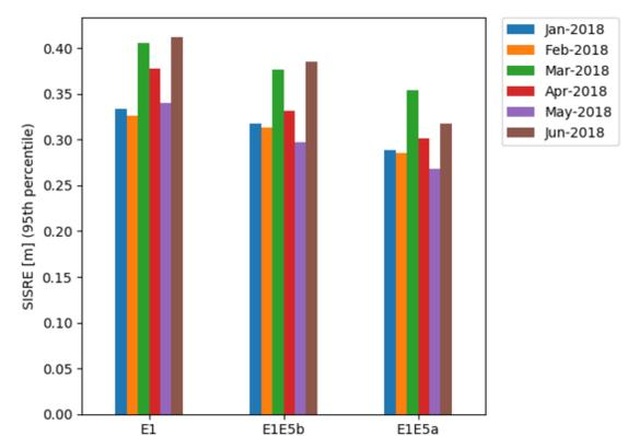
Figure 3 : Signal combination for Galileo single- and dual-frequency users, whereby E1 and E1/E5b users apply I/NAV and E1/E5a users F/NAV navigation message
