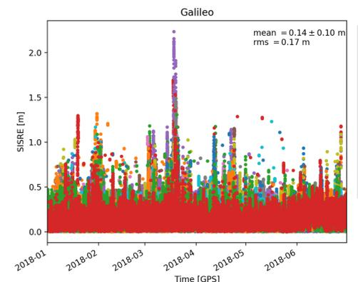
Figure 1 : Global average SISRE for Galileo signal combination E1/E5a and use of F/NAV navigation message
