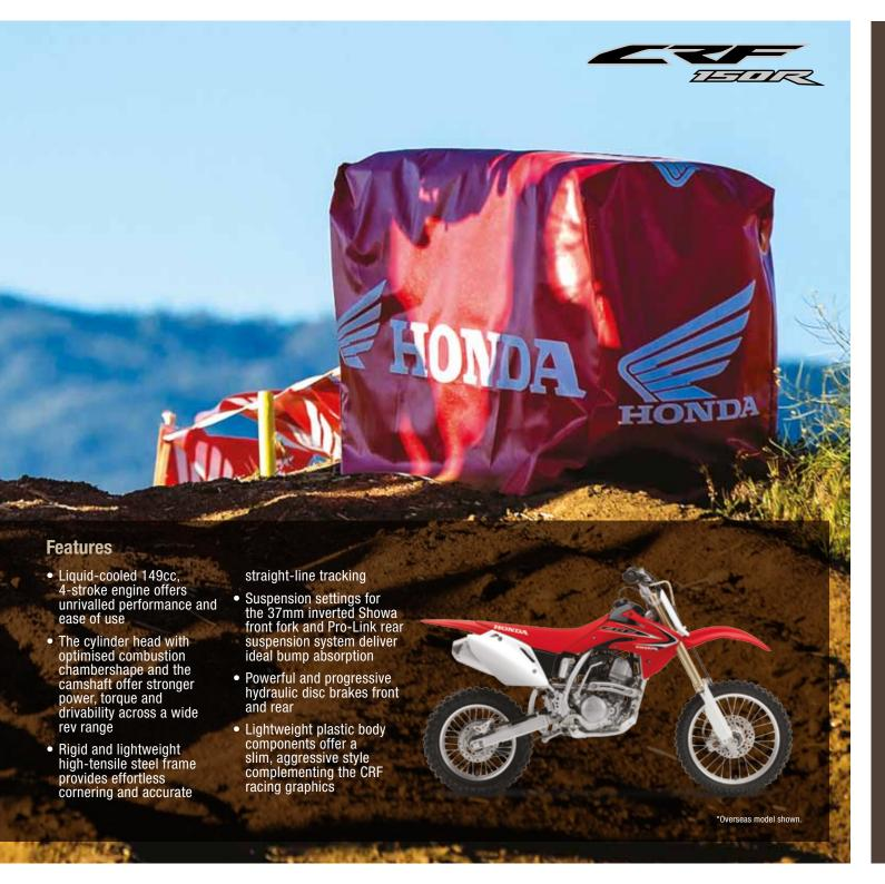
Engine Type 149.9cc, liquid-cooled single cylinder
