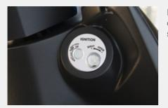
Key hole is covered by lid to prevent motorcycle theft. Easily access the under-seat compartment using the main ignition keyhole, eliminating the need to remove key to open seat compartment.
