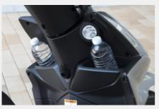
Both left (600 ml) and right (500 ml) storage compartments provide ample room together with covered key functionality layout above the right pocket.
