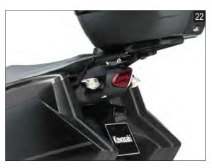
\* Large under-seat storage space has room for compact rain gear or other small items. Tool kit is affixed to the bottom of the seat.
