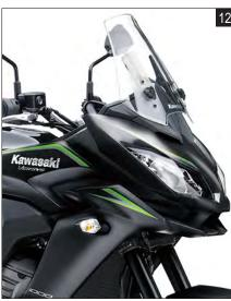
\* Chin spoiler below the twin headlamps helps direct wind around the upper cowl for increased stability at highway speeds as well as increased comfort for the rider. (Photo 13)
