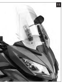
\* Wind passages between the upper and side cowls were aerodynamically designed to help reduce air resistance while managing airflow for increased wind protection and comfort. (Photo 12)
