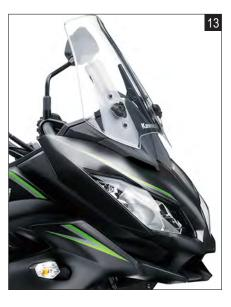
\* Air intake between the headlamps at the cowl bottom routes fresh air into the cockpit to relieve the effect of negative pressure at high speeds. This helps prevent helmet buffeting. Fresh air is also routed to the inside of the cowl to help keep parts that generate heat cool.
