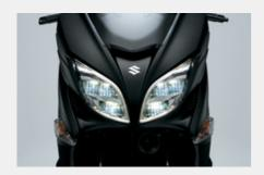
The slim, elegant styling of the new nose features sharply styled dual LED headlights with integrated LED position lights and turn signals mounted beneath. The overall effect creates a cleaner and lighter looking front end that is instantly recognizable as belonging to the BURGMAN family.
