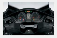
Large, easy-to-read analogue speedometer and tachometer dials flank a digital display that shows an odometer, dual trip meters, fuel gauge, coolant temperature indicator, average fuel consumption meter, ambient temperature indicator, freeze indicator and clock. Also included is Suzuki's Eco Drive Indicator, which come on when the vehicle is operated in a fuel-efficient manner and may help riders learn techniques to better economise on fuel.
