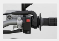
Push-button electric start fires up the bike consistently, powered by a small and reliable battery.
