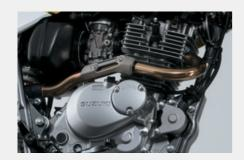
The DR200S's 199cm3 single-cylinder air-cooled four-stroke engine provides just the right amount of torque and horsepower to power your ride.
