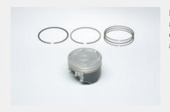
In order to further improve overall fuel efficiency and emissions control, the V-Twin engine adopts two innovations: resin coating on the piston skirt for minimised friction between the cylinder and piston, and a special L-shaped piston ring for enhanced sealing performance and blow-by gas reduction.
