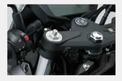
Front forks are equipped with a new Preload Adjuster, allowing you to set suspension firmness for exactly the way you want to ride.
