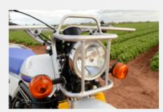
Heavy-duty headlight protector is also capable as a carrier for light loading. Sturdy steel protectors for brake and clutch levers are also fitted as standard eqipment.
