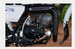
123cc, piston-reed-valve 2-stroke, air-cooled engine that produces abundant usable torque with excellent fuel economy.
