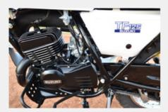
Engine bar and plate protect the bottom of the engine.
