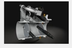
Suzuki Dual Throttle Valve (SDTV) induction system is enhanced by the 32-bit engine control unit that instantly delivers the optimum fuel-air mixture and power output. The system – it's the same design used in Suzuki championship-winning GSX-R sportbikes – delivers seamless throttle response while boosting fuel efficiency and delivering strong torque.
