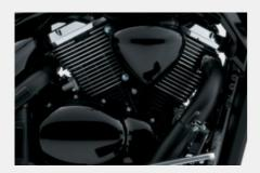
90 cubic-inch (1462cm3) long-stroke V-Twin engine powers the SUZUKI BOULEVARD C90T cruiser. Using features found only in Suzuki motorcycles, this powerplant makes massive torque while also delivering fuel-efficient, usable power. Yes, it's the most powerful in its class, but it's more than just muscular. This powerplant delivers the best blend of power, efficiency and torque for comfortable, long-range cruising.
