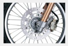
The lightweight 290mm front floating-disc brake with dual-piston caliper and the 240mm rear disc brake with twin-piston caliper together provide reliable stopping power with excellent feel at the lever.
