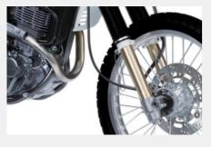
The front fork combines the best features of conventional and inverted designs: smooth and progressive action on a variety of road or trail riding surfaces. Large diameter, thin-walled tubes reduce unsprung weight while maintaining high rigidity with minimal below-axle extension. A link-type rear suspension with piggyback-style shock absorber and adjustable compression damping provides stable performance over any terrain.
