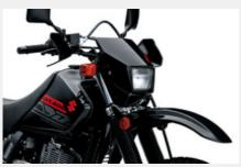
Bright 60/55 watt halogen headlight; handlebar-mounted handguards and special design tires with on/off-road tread pattern fitted to 21-inch front and 17-inch rear wheels.
