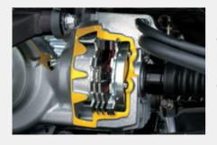
Dual front hydraulic disc brakes with large 200mm discs and lightweight calipers provide maximum brake pad surface area for increased stopping power and outstanding durability. Working together with a sealed multi-plate rear brake system, with a clutch-type design, provides high durability, offers reduced unsprung weight, and is almost maintenance free. Its sealed design ensures strong, effective braking over nearly any kind of terrain or conditions.
