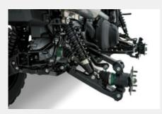
Ride quality and manoeuvrability especially over rough terrain has been improved with the addition of nitrogen charged shock absorbers, featuring 5-way spring preload adjustment all round. The independent double A-arm front suspension features 170mm of wheel travel whilst up back the fully independent, A-arm/I-beam features 195mm of wheel travel.
