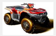
All new bodywork and styling featuring sharper lines with well-defined angles. The high-clearance fenders offer great protection for the rider from flying debris. Australian-spec KingQuad ATVs also come standard with overfenders for extra protection. The refined panels simplify maintenance needs, such as checking oil level, fuel filter and air filter servicing.
