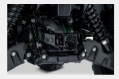
Towing capacity has been increased by 33% from 450kg to 600kg. Additionally the trailer hitch mount has been changed from a plate type to a receiver type allowing customers to easily change hitch and ball types when required.
