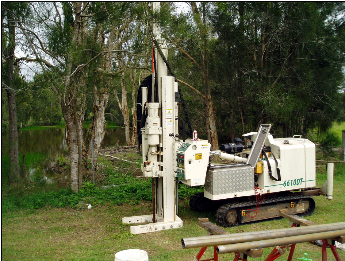
Plate 1. Geoprobe model 6610DT track-mounted coring machine
