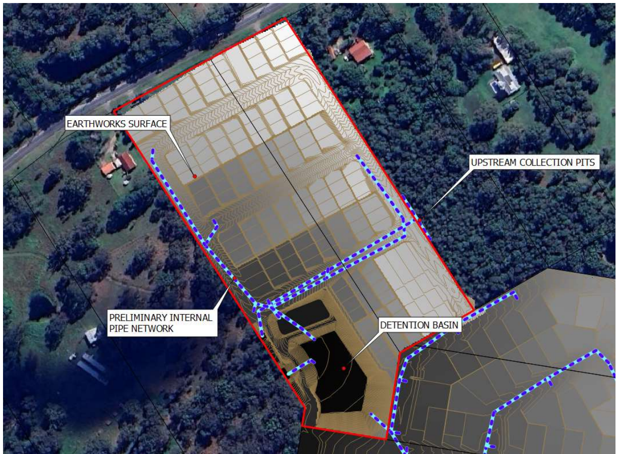
Figure 3-7 – Post-Development Model Modifications
