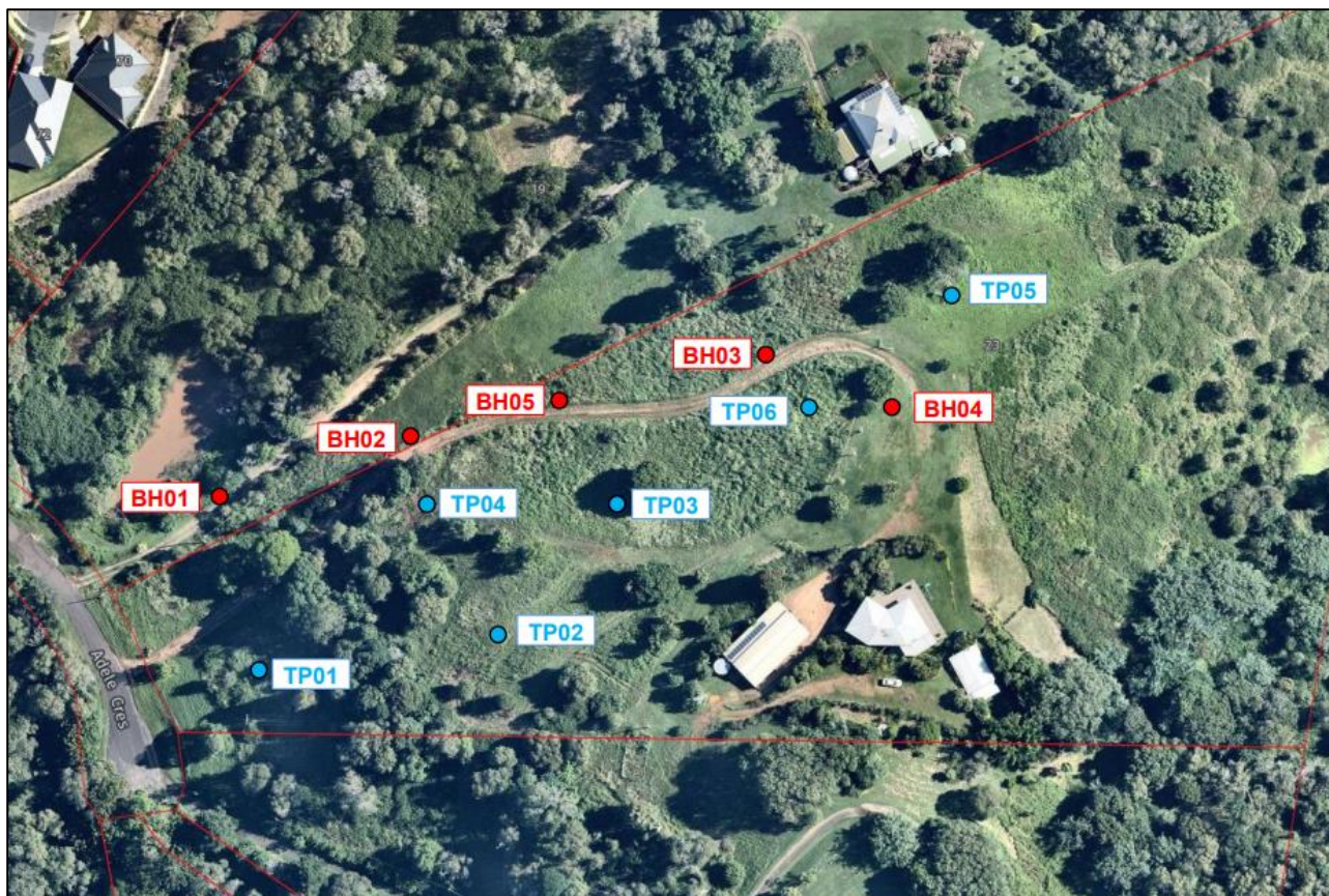
Figure 2.4 Borehole and Permeability Testing locations (Courtesy: Soil Surveys)
