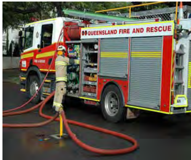
Figure 2 – Use of Hydrant System
