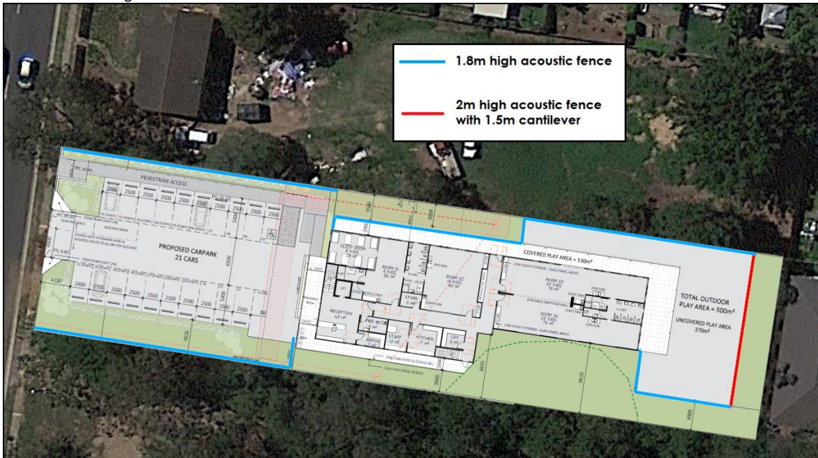
Plate ES1: Showing recommended acoustic barriers
