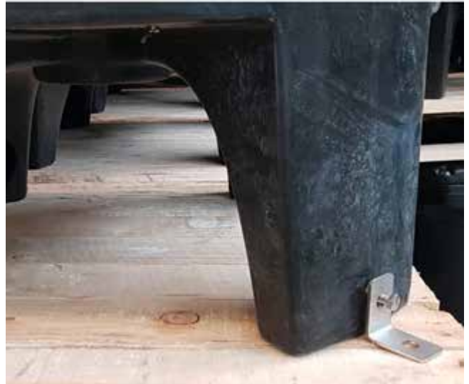
Figure 4 - Bolting the feet
