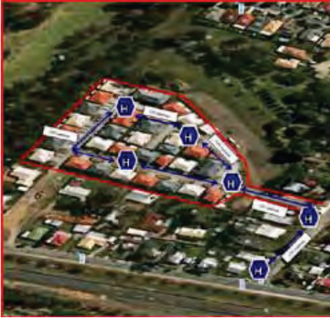
Figure 6 – Hydrant System design to minimum standards
