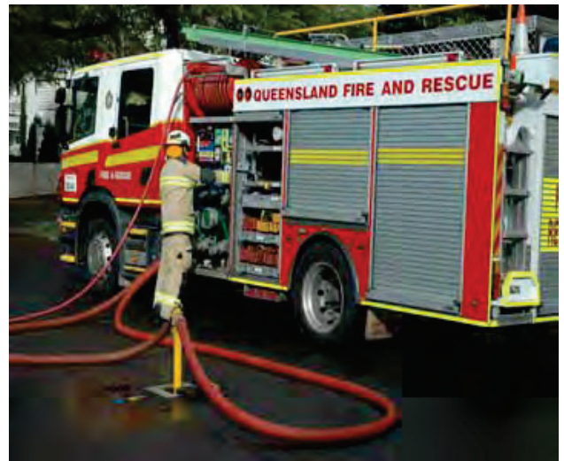
Figure 2 – Use of Hydrant System
