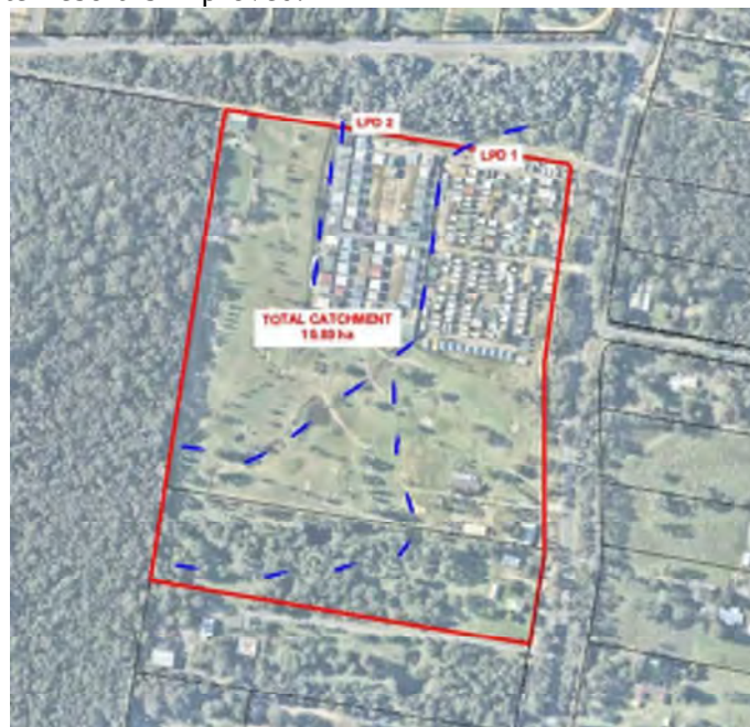
Figure 2-1 – Pre-Development Flow Characteristics & Lawful Points of Discharge
