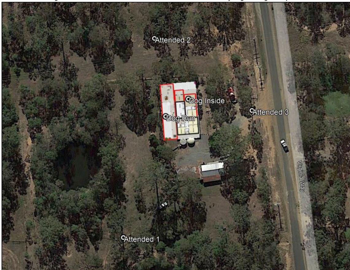
Plate 4.2: Showing the attended noise measurement location and location of dogs during survey.
