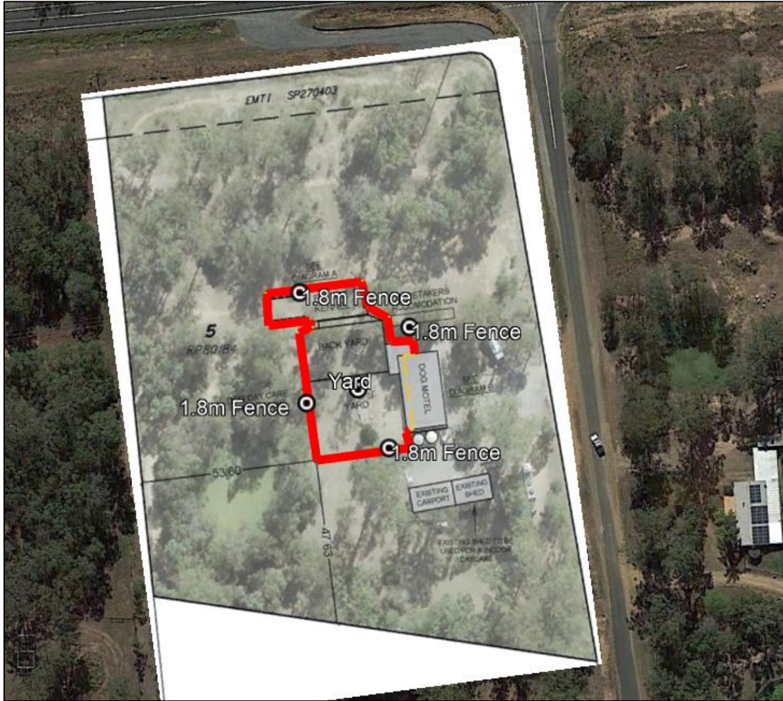
Plate ES1: Showing proposed location of acoustic fence marked red on Plans, at 1.8 metres above ground level.
