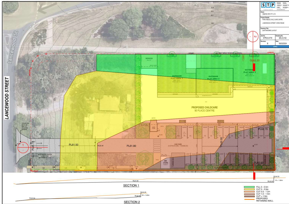
Figure 3.5 –Preliminary earthworks layout
