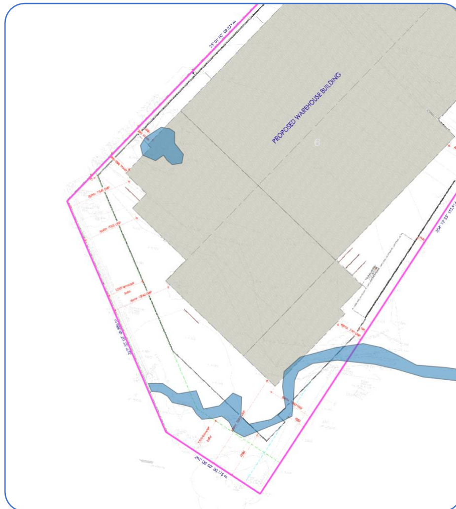
Figure 9.1 Waterway Flow Path and Development Impacts
