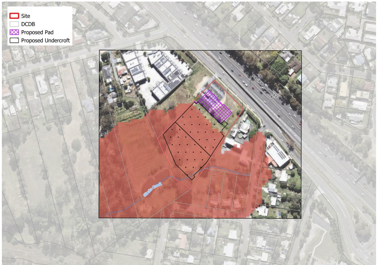
Figure 21 High Flow Area (Shaded Red) in context to the Proposed Undercroft and Fill Area
