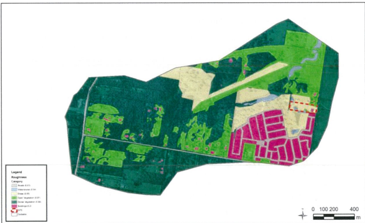
Figure 3-3 TUFLOW Model Hydraulic Roughness
