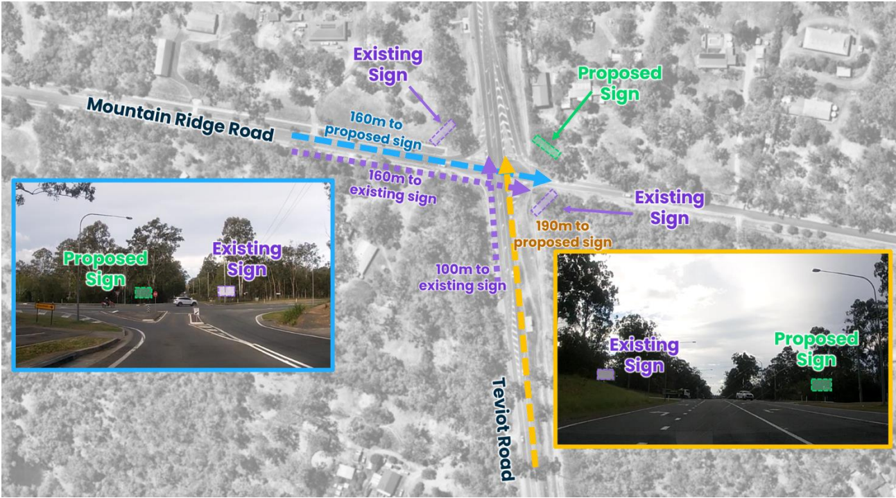
Figure 2. Available Sight Distance to Proposed Sign and Existing Signs
