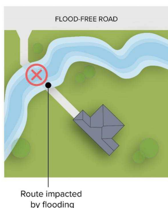
Figure 9.3.2.3.2 - Non-compliant dwelling with no flood-free vehicle route
