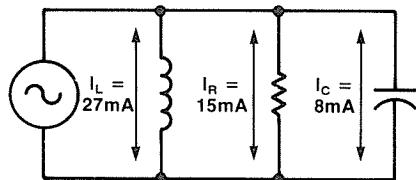
2. Draw power phasor diagrams for the circuit in problem 1. Calculate the value and sign of the phase angle.
