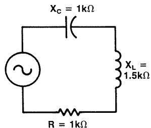
2. Draw a phasor diagram for this circuit showing power and voltage phasors.
