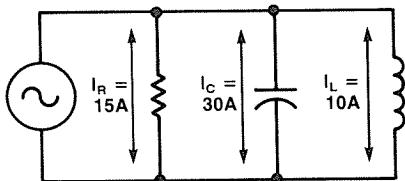
3. Calculate the value and sign of the phase angle in the circuit of Problem 1.
