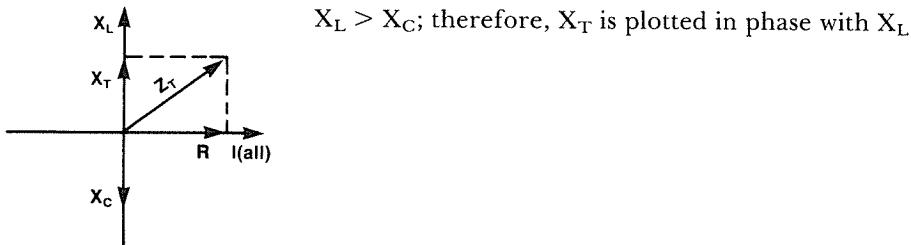
2. Draw voltage phasor diagrams for the circuit in Example 1. Calculate the value and sign of the phase angle.
