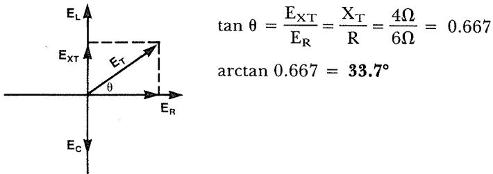
The angle is rotated counterclockwise; therefore, the sign of the angle is positive.
