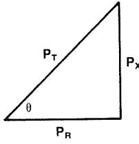
$$\begin{aligned} I_T &= \sqrt{I_R^2 + I_X^2} \\ &= \sqrt{I_R^2 + (I_L - I_C)^2} \end{aligned}$$
