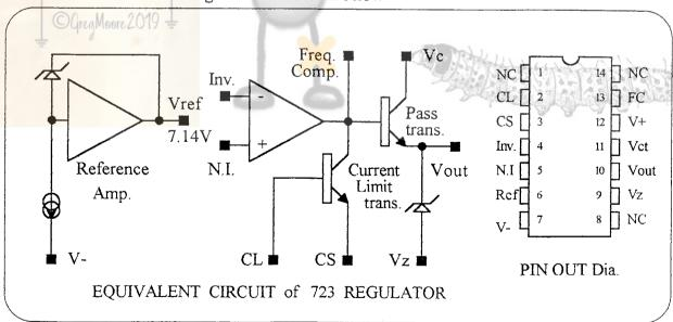
The maximum input voltage is 40V and the chip can be used to regulate between 2 to 37V using selected circuits. The zener diode Vz is to allow the regulator to operate as a high voltage floating supply or to produce negative voltage using a suitable circuit.
