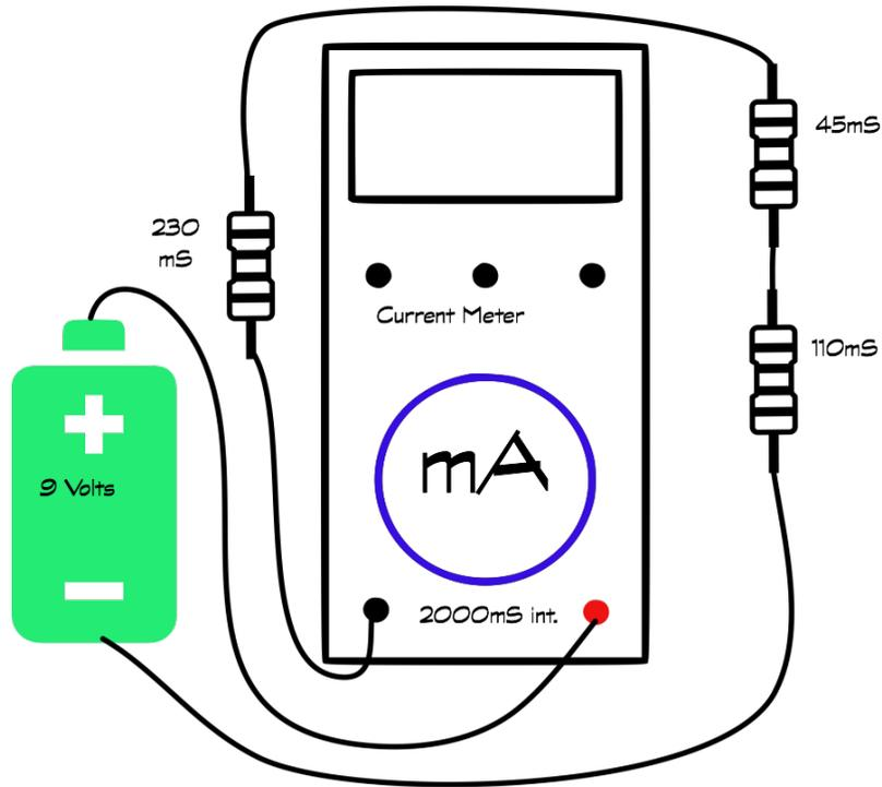
Wires are all 45S/Metre conductance and have a total wire length of 33cm.
