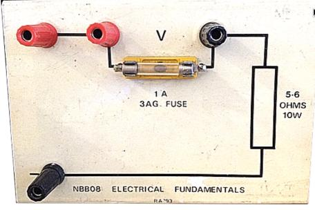
Most all circuits involving higher current levels use a fuse such as this or some other form of current limiting.
