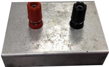
This is a component holder for our Lab. You will place a 100 Ohm resistor in one, and the 68 Ohm resistor in the other.
