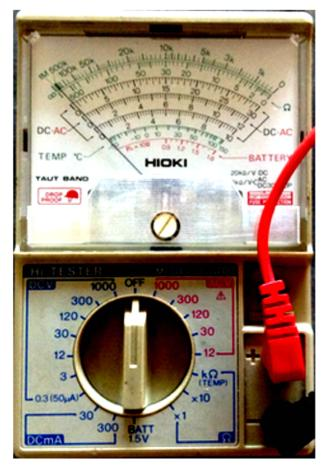
This is a multi-meter. It can do many different measurement functions. Volts, Amps, Ohms. Really versatile and not an old out-dated appliance, so please do not call it that. Every test item has it's place in electronics work.
