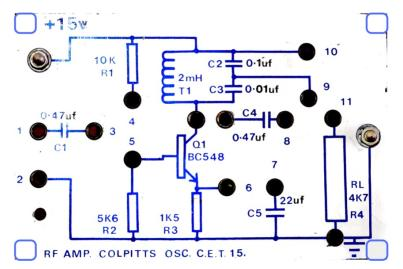
hand side of C4 to the collector of Q1. What happens to the output waveform and voltage? Explain.
