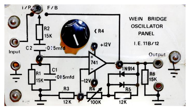
ien Bridge on the top, excuse my predecessors for the bad spelling! Run the calculations from the video and determine the operating frequency. What is the purpose of the back to back diodes? And the  $12k\Omega$  resistor? Given that R3 is  $12k\Omega$  what should the feedback resistance be for oscillation?
