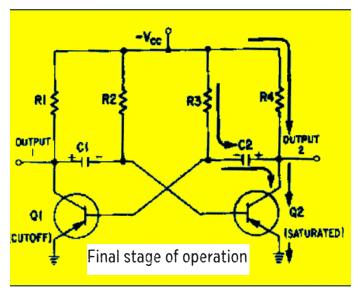
final stage of operation, the circuit is the mirror image of the first stage of operation. In the circuit above the left side of capacitor C2 becomes more negative at a rate determined by the time constant R3C2. As the left side of C2 becomes more negative, the base of Q1 also becomes more negative. When the base of Q1 becomes negative enough to allow Q1 to conduct, Q1 will again go into saturation. The resulting change in voltage at output 1 will cause Q2 to return to the cutoff state.
