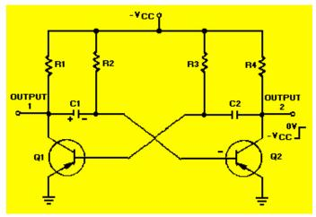
on the right side on capacitor C1 has caused Q2 to conduct. Now the following sequence of events takes place almost instantaneously. Q2 starts conducting and quickly saturates, and the voltage at output 2 changes from approximately -VCC to approximately 0 volts. This change in voltage is coupled through C2 to the base of Q1, forcing Q1 to cutoff. Now Q1 is in cutoff and Q2 is in saturation. This is the circuit situation shown in figure on the next page. Notice that in the
