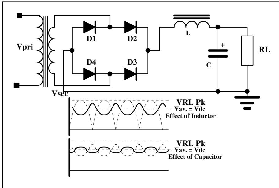
2. *Pi ( $\pi$ ) filter* - By following a capacitor filter with a choke filter, a  $\pi$  filter is constructed which allows for a greater output voltage but with the advantage of much improved filtering of the ripple component of rectification. The diagram on the right shows the basic circuit. This type of filter was once very popular but is only found in
