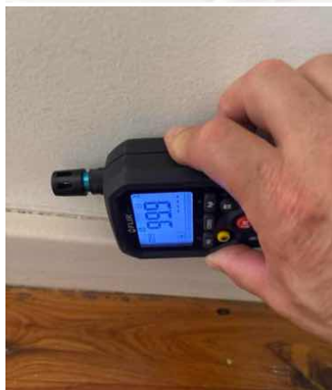
Example of elevated moisture r readings in walls, photo from the hallway near the shower
