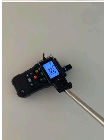
Example of elevated moisture r readings in walls, photo from the hallway near the shower
