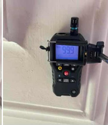
Example of elevated moisture r readings in ceilings, photo from the family / meals
