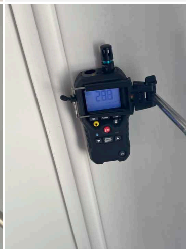
Example of elevated moisture readings in ceilings, photo from the office / study
