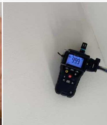
Example of elevated moisture readings in ceilings, photo from the office / study
