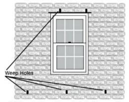
Weep holes allow air into the cavity and moisture to drain out
