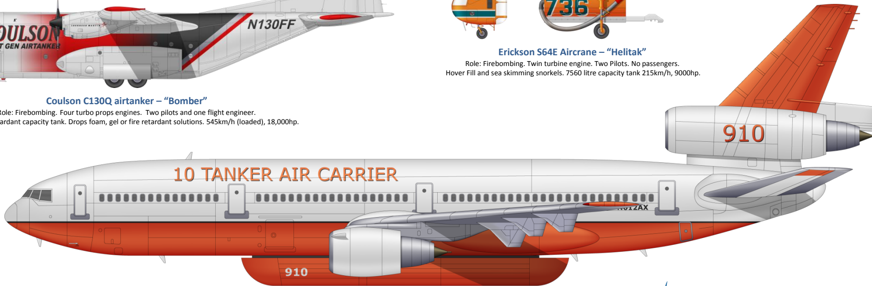
McDonnell Douglas DC10-30 – “Bomber” Role: Firebombing. Three turbo fan engines. Two pilots and one flight engineer. 43,900 litre retardant capacity tank. Drops foam, gel or fire retardant solutions. 650km/h (loaded), 73,000kg thrust.
