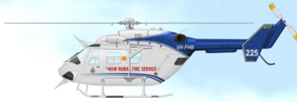
MBB/Kawasaki BK 117 – “Helitak” Roles: Fire crew insertion, firebombing, transport, utility. Twin turbine engine. Eight Passengers. 270kg, 75m winch. 900 litre capacity bucket. 215km/h, 1500hp.
