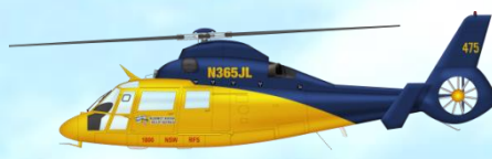
Eurocopter AS365N2 Dauphin – “Helitak” Roles: Fire crew insertion, firebombing, transport, utility. Twin turbine engine. Eight Passengers. 270kg, 100m winch. 1025 litre capacity bucket. 260km/h, 1500hp.
