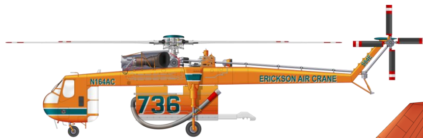
Erickson S64E Aircrane – “Helitak” Role: Firebombing. Twin turbine engine. Two Pilots. No passengers. Hover Fill and sea skimming snorkels. 7560 litre capacity tank 215km/h, 9000hp.
