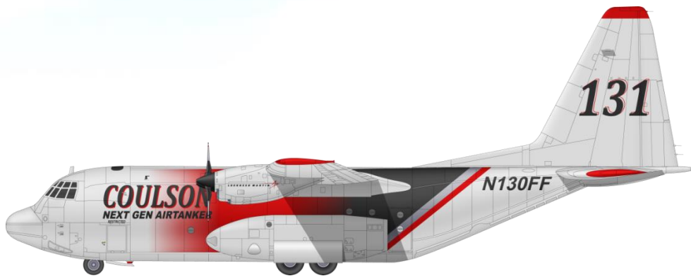
Coulson C130Q airtanker – “Bomber” Role: Firebombing. Four turbo props engines. Two pilots and one flight engineer. 15450 litre retardant capacity tank. Drops foam, gel or fire retardant solutions. 545km/h (loaded), 18,000hp.
