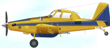
Air Tractor AT802F – “Bomber” Role: Fire bombing. Single engined, turbo prop air tanker. 3200 litre capacity. Drops water, foam, gel or fire retardant solutions. 350km/h, 1600hp.
