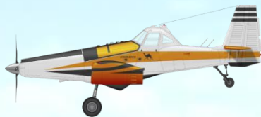
PZL M18T (Hubler) Dromader – “Bomber” Role: Fire bombing. Single engined, turbo prop air tanker. 2375 litre capacity. Drops water, foam, gel or fire retardant solutions. 230km/h, 1000hp.
