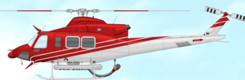
Bell 412SP – “Helitak” Roles: Firebombing, fire crew insertion, transport, utility. Twin turbine engine. 10 passengers. 270kg, 75m winch. 1400 litre capacity belly tank. 225km/h, 1800hp.
