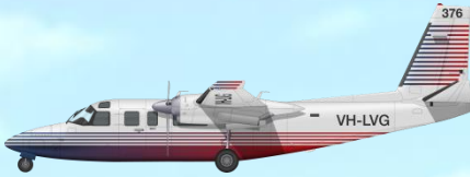
Rockwell Turbo Commander 690B– “Birddog” Roles: Supervision, reconnaissance, transport, utility. Twin turbine engine, high wing. Five passengers. 500km/h 1430hp.
