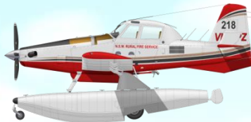
Air Tractor AT802F Fireboss – “Bomber” Role: Firebombing. Amphibious, single engined turbo prop air tanker. 3200 litre capacity. Scoops water from lakes and rivers, adds foam, gel before dropping. 275km/h, 1600hp.
