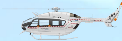
Eurocopter EC145 – “Helitak” Roles: Fire crew insertion, firebombing, transport, utility. Twin turbine engine. Eight Passengers. 270kg, 91m winch. 910 litre capacity bucket. 220km/h, 1500hp.
