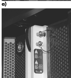
a) b) Fig. 42: J-SUB and J8/J12 Ground stack Assembly of the Flying frame
