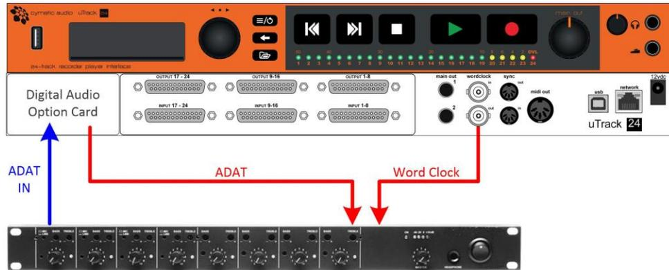
In this most common setup the uTrack24 is clock master and creates its own sampling rate. In recording mode the sampling rate is defined in the “Recording” menu, and in playback mode it is the song’s sampling rate.
