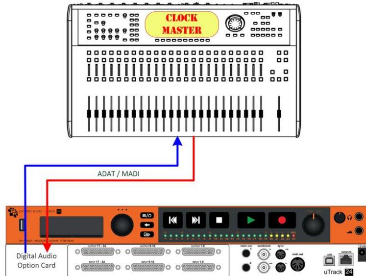
With a digital expansion card installed in your uTrack24, it is possible to directly synchronize your unit to a MADI or an ADAT input signal, without the need for an additional word clock cable.
