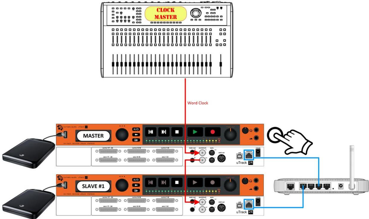
If you need to synchronize a sync group to an external clock master, it is mandatory distributing the clock to all uTrack24 units. In the example shown above, the master word clock is fed to the first uTrack24 which in turn provides its word clock output to the next uTrack24. Both units have the clock source set to Wordclock.
