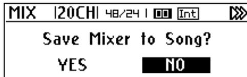
When playing back a song or when it is preloaded, the song’s mixer setting is loaded. The mixer parameters can be changed if needed. To save the changed mixer parameters to the song, click on the Menu button. If the mixer is changed and you press the back button , you will be prompted to save the mixer settings.
