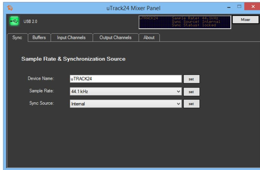
**Device Name:** The device name field controls what device name will appear in your DAW software. The default name is “uTrack24” but it can be modified to the name of your choosing.
