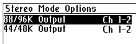
When playing back a stereo audio file, the uTrack24 allows selecting a pair of rear-panel outputs on which the file will be played out.
