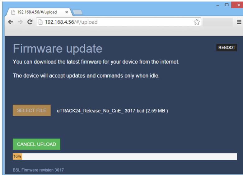
After the image is successfully updated, the browser shall ask to reboot the device. Click the green “REBOOT” button. The connected uTrack24 will reboot which concludes the update process. The screen will show the version number of the updated firmware.
