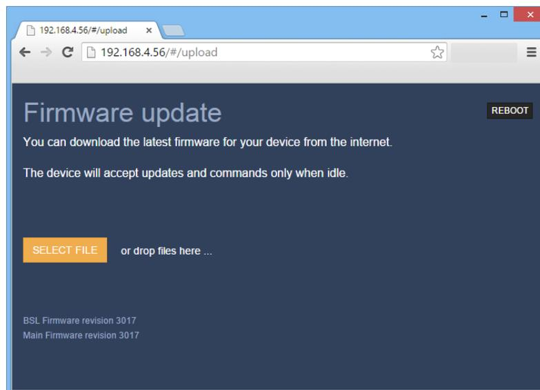
Drag and drop the firmware update file onto the orange SELECT FILE button. Alternatively click the SELECT FILE button and select the file with the file browser that opens.
