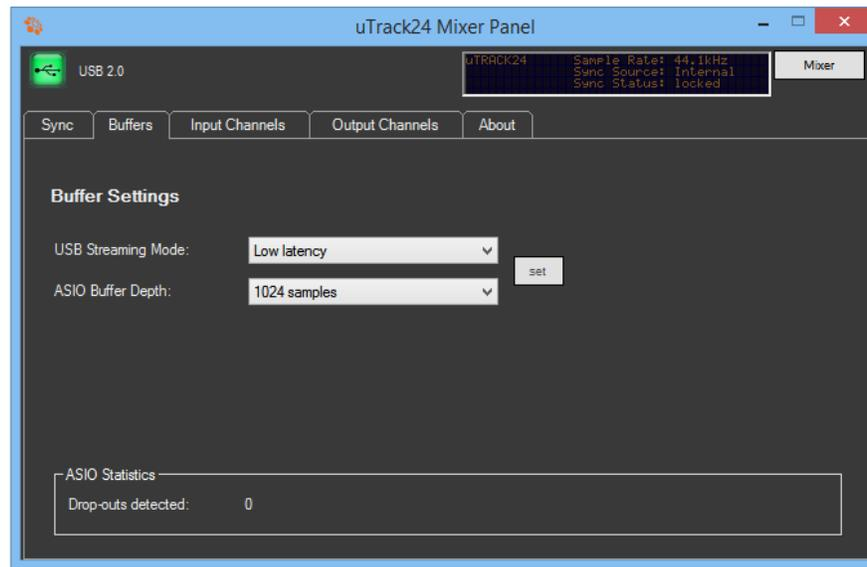
The control panel's buffers screen allows adjustment of the ASIO buffers used by your ASIO compatible software.
