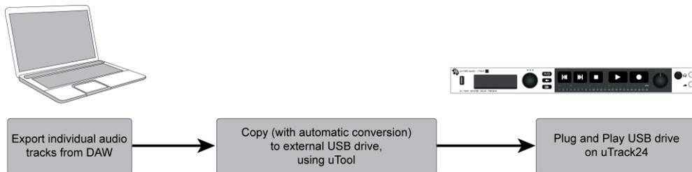
When playing back a take, the uTrack24 performs seamless transitions from the end of one “chunk” of multi-channel audio to the beginning of the next one. Multiple chunks inside a take are played back as if they were one long take.
