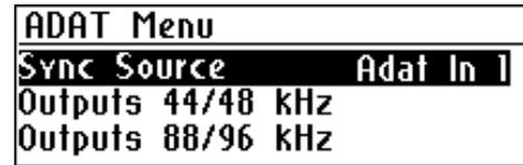
**Sync Source:** Selects which of the 3 ADAT input would be used as the sync source. The clock source should be set to Digital I/O to have the device synced to the ADAT card.
